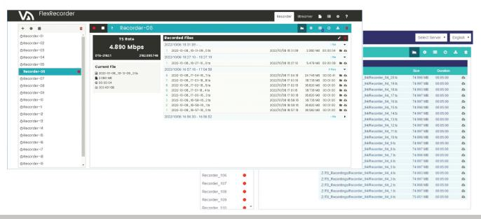
The Village Island FlexRecorder is a 24/7 recording system, that can capture to files any type of input, such as RF, ASI, or IP. The system can be scaled to record any number of input streams, over any length of time with the addition of servers and interface cards. Retrieval of archived TS data is done through the extractor interface, allowing the user to search through the archive and download the desired segment as a single file.
