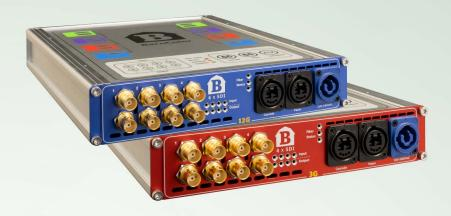
Each BarnColor SDI pair handles up to 8 signals (4 forward and 4 returns). 4 different colors can be cascaded / daisy chained up to 32 x Signals (16 forward and 16 returns). Can be combined with any models in different colors.
