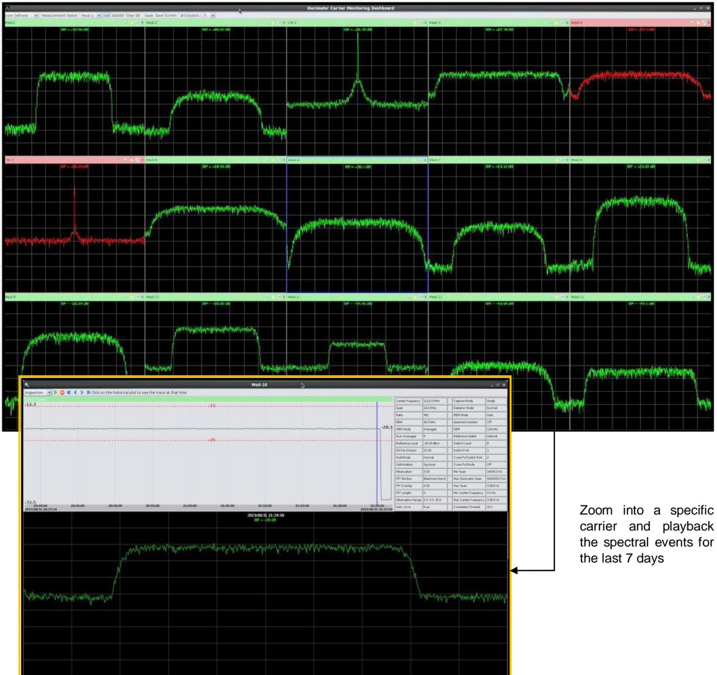
Zoom into a specific carrier and playback the spectral events for the last 7 days
